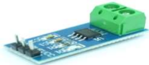
Gambar 13. Sensor Arus ACS 712
