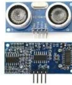
Gambar 2.6 Sensor Ultrasonik
