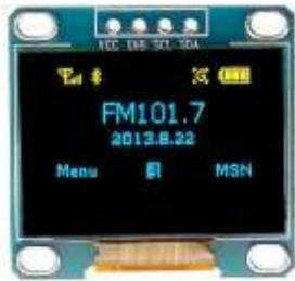
**Gambar 7. OLED Display I2C**
